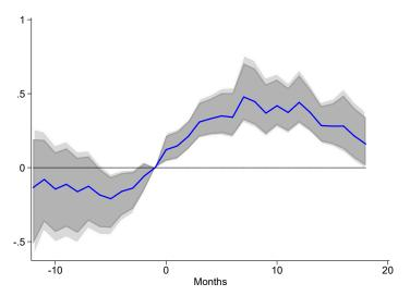
Local projections response of log output per hour worked to 1% shock to aircraft demand, instrumented with the ("leave one out") production of broad aircraft of the same broad type. Includes month and plant × model (production line) fixed effects, 6 monthly lags ofcapital per worker. 90% and 95% Finlay-Magnusson weak-instrument robust standard errors shaded. Montiel-Olea and Pfluger F-stat at 12-month horizon = 40. Return
